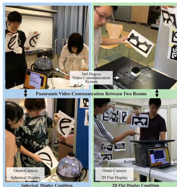
図 1: The 360 ° video communication systems. Local room and remote room are connected by two different types of 360 ° video communication systems, which are combining a omnidirectional camera with a spherical display(upper left)(lower left) or with a horizontally placed 2D flat display(upper right)(lower right).
