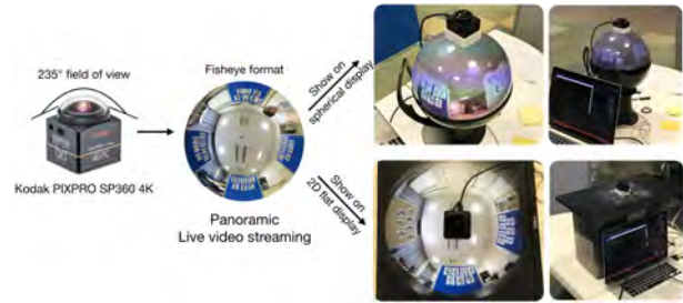
Fig 2: The diagram of the panoramic video system. The input of the system is from the Kodak camera. The output is either on the spherical display or the 2D flat display.
