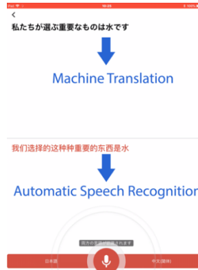
Fig. 2. The interface of the real-time language support tool. In this figure, a Chinese utterance is translated to Japanese (“The most important item we chose was water.”)
